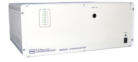
The PSA S665S200 product range is utilised when numerous sample streams need to be monitored, or when zero and span gases need to be diverted to a probe. The unit consists of a Mass Flow Controller plus a number of 3-way Teflon Switching Valves. A sample pump is supplied with the unit. The Stream Selector can be configured for positive or negative flow applications.
